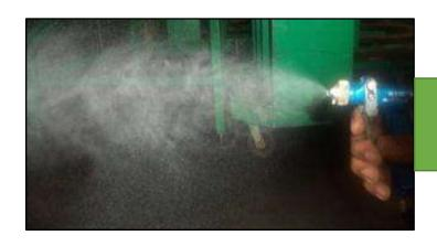
Fly loss reduction Nozzle diameter from 1mm to 0.5
