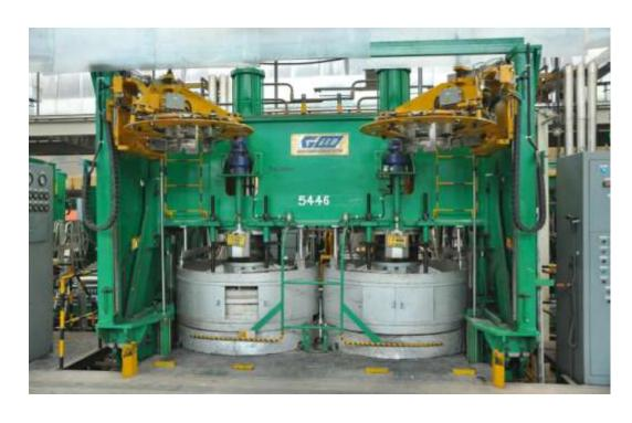
Platen Type Curing Press in CTP
